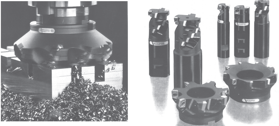
Figure 2.16: A face milling operation and various inserted milling cutters. Source: Mitsubishi Materials.
